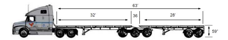
1. **Open Flats** for over-dimensional loads or standard capacity loads of up to 68,000lbs (Maximum payloads vary from State to State)
